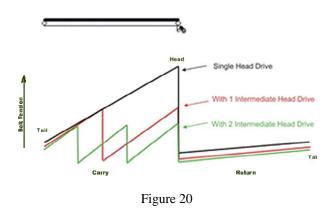
By splitting the power into two locations (red line), the maximum belt tension is reduced by almost 40% while the total power requirement remains virtually the same. A much smaller belt can be used and smaller individual power units can be used. To extend the example further, a second intermediate drive is added (green line) and the peak belt tension drops further.
