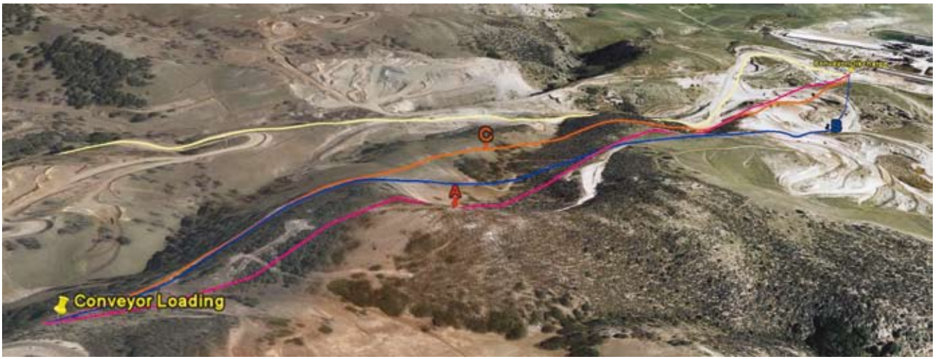
Figure 5. Three possible conveyor routes.
