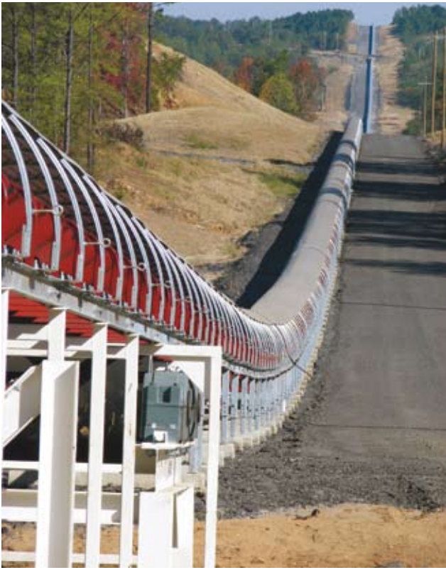
Figure 2. A belt conveyor is adaptable to difficult terrain. Photo Courtesy Continental Crushing and Conveying
